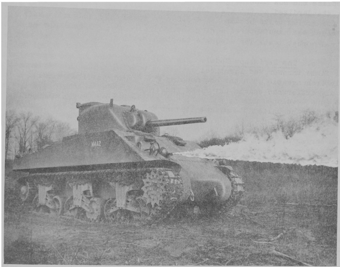
Figure 6. The M3-4-3 Mechanized Flame Thrower—an Auxiliary Type.
